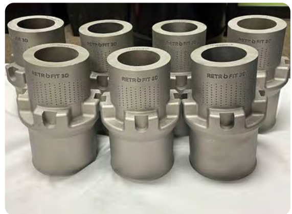
Completed choke valve trims printed in Inconel® 718 on six separate Velo3D Sapphire printers across three continents.
