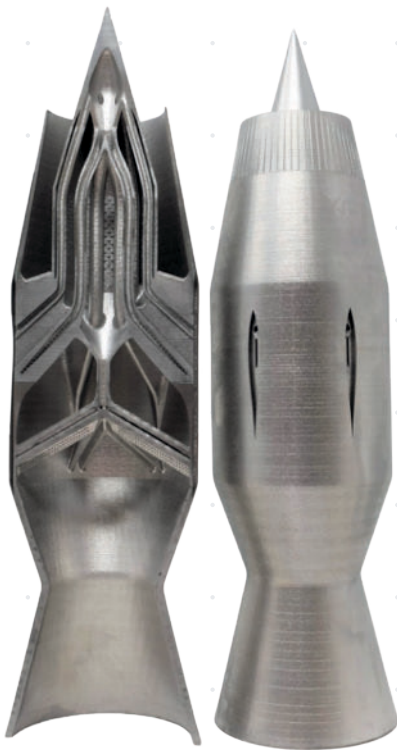
Hypersonic Ramjet model featuring integrated complex internal flow channels, printed on a Velo3D Sapphire printer.
