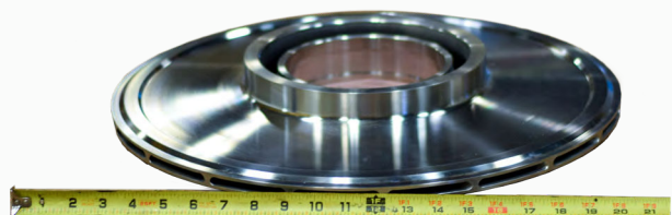
View of completed 483 mm shrouded impeller printed on a Velo3D Sapphire XC. For scale, the impeller is bigger than a typical NY-style pizza (typically 18”).
